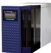
Hydrogen G200/G400/G600/G600-HP are bench-top generators that utilize a Proton Exchange Membrane (PEM) cell stack and desiccant dryer to produce ultra high purity (UHP) hydrogen for laboratory applications. These systems are capable of sensing demand and adjusting production rate, while maintaining quiet operation
