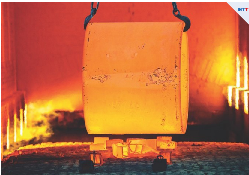
Hydrogen scavenges oxygen, counteracting minor furnace leaks.
