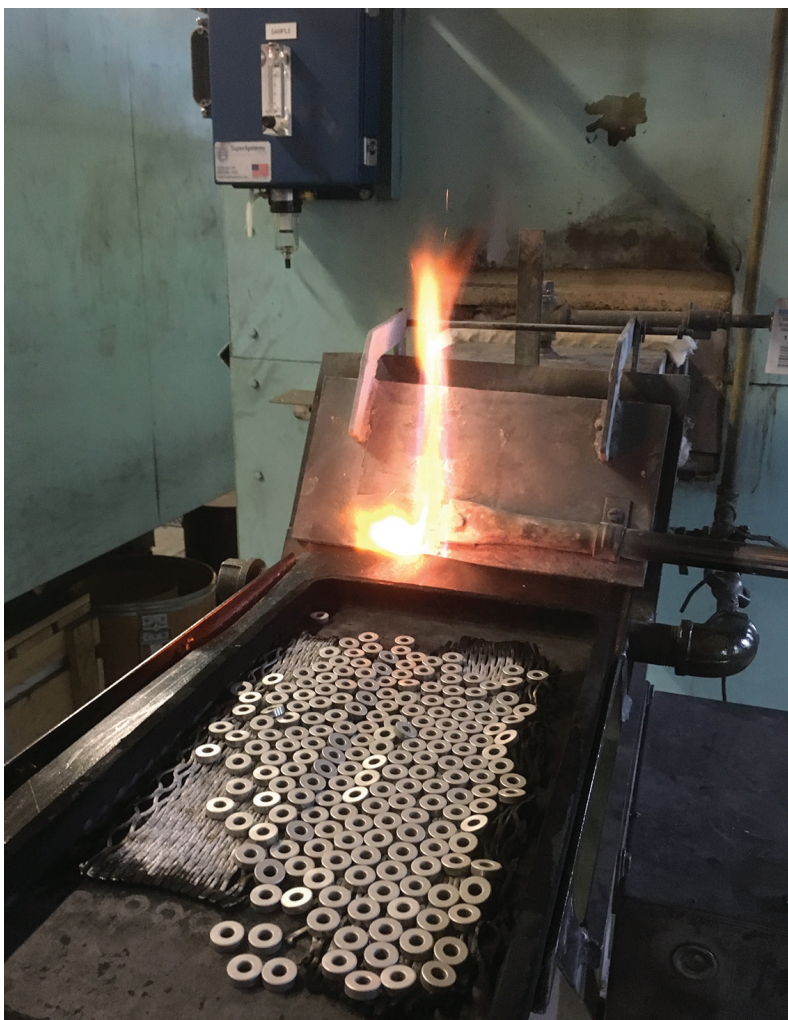
Hydrogen cleans part surfaces to enhance processing results.
