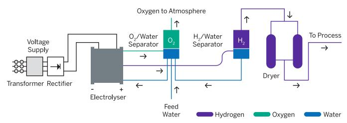
Electrolysis is the process of splitting the water molecule into hydrogen and oxygen using electricity. The inputs to this process are simply feed water and the current supplied to the electrolyser.
